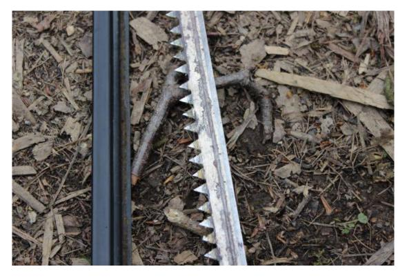
The raker blade is specifically designed for cutting green wood with every third or forth notch having a V shape.
